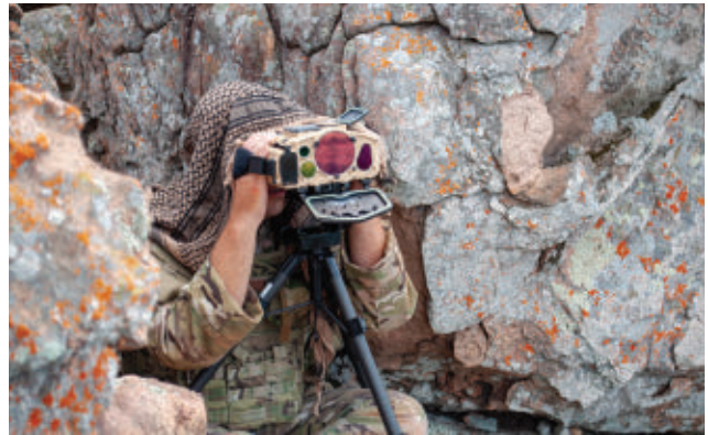
The Joint Effects Targeting System (JETS) from Leonardo DRS is a hand-held target location system that enables forward observers to carry out necessary reconnaissance on targets and communicate the coordinates instantaneously to the network of maneuver commanders.
